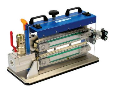
BDJ Hydro Chain Cable – the most powerful, chain blowing machine for classic fiber optic and copper cables. Machine has failure-free hydraulic engines and cable feeder on roller chains. It is driven from a hydraulic power pack (included). Machine has a solid construction, high quality feeder and the power of hydraulic motors that allows blowing cables over a distance of up to 2,5 km.
