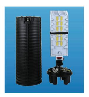
53703001 fiber optic splice closures are specially designed to protect joints of optic cable. Excessive fibers can be stored in storage baskets behind the splice trays. The optical fibers are fusion on sides of the tray.
