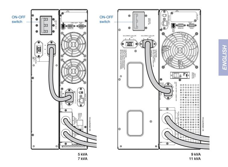
Connection of multiple batteries
