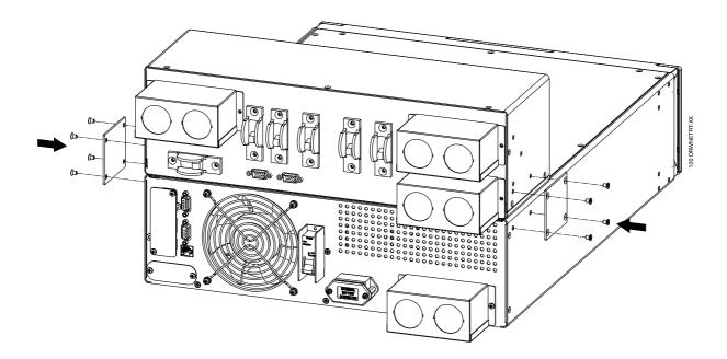
7.1.2 Fixing BY-PASS to UPS for vertical installation
