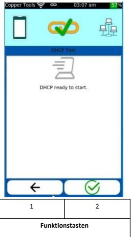
In the **DHCP Test**, LinkXpert checks whether the device can be assigned an IP address by the network and whether other information such as DNS server address and address range is transmitted.
