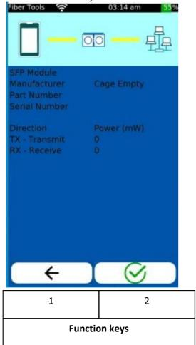
In the **TX/RX** the transmit (TX for Transmit) and receive values (RX for Receive) of the SFP module as well as information about the SFP module are read out.
