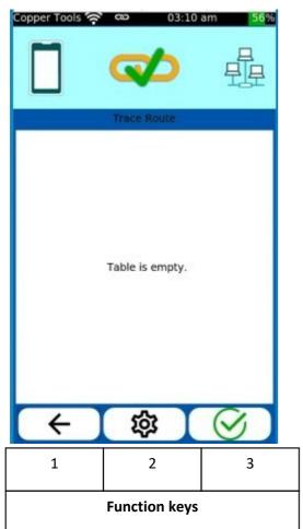
In the **Traceroute** test, LinkXpert shows intermediate stations that IP packets pass through until they arrive at a defined destination.
