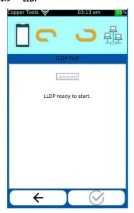
In the **LLDP** test LinkXpert lists LLDP responses of the connected switch.
