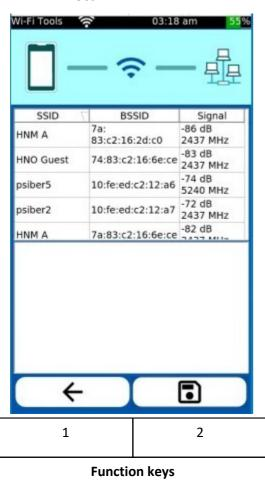
In the **WiFi Scan** test, LinkXpert M3 scans the 2.4 and 5 GHz bands for access points and lists the access points.
