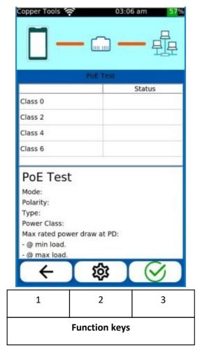
The **PoE Test** tests the ability of network switches to provide remote power according to IEEE802.3.
