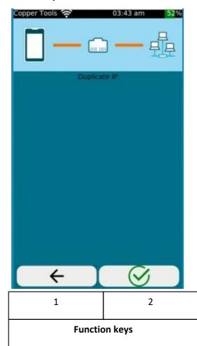
In the **Duplicate IP** test, LinkXpert scans the network for devices on the network that use the same IP address.
