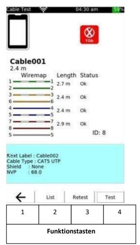
In the wiring test module, the device displays the wiring diagram with lengths.
