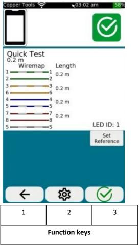
The wiring diagram is given per pin, the length per pair. The shortest length is shown in the report as link length.
