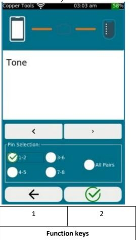
The built-in tone generator is compatible with analog cable locators such as Softing CP15. This menu is only accessible in the Tools module.
