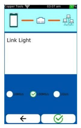
To identify the link LED on the switch, LinkXpert can flash the link LED of the switch port. To do this, LinkXpert must be connected to a switch via the copper or fiber interface.
