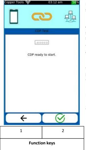
In the **CDP** test LinkXpert lists CDP responses of the connected switch.
