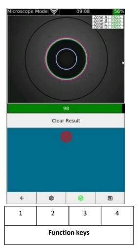
In the **microscope t**est the surface of fiber optic connectors and issue a good / bad statement according to IEC standard.
